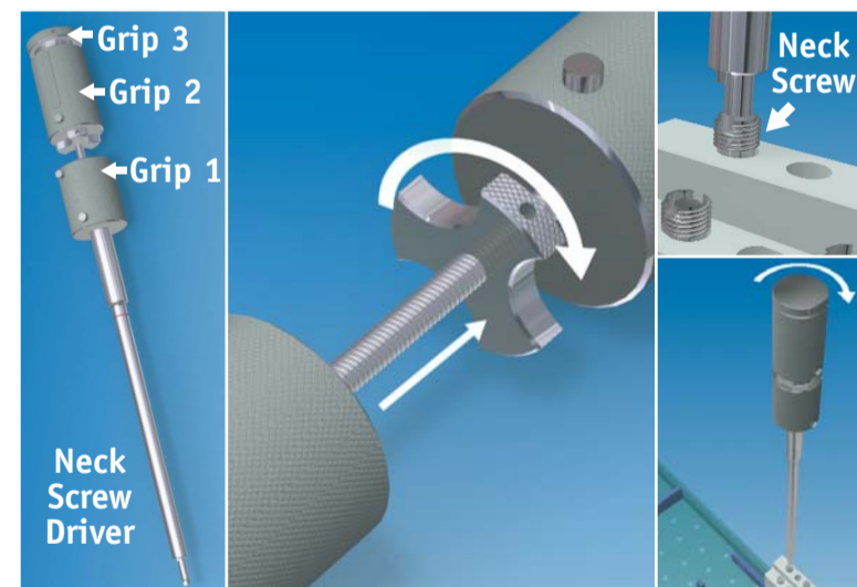
18 Attach Neck Screw to Neck Screw Driver
