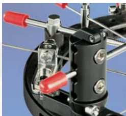
The Sheffield Clamp has a strong base to reduce cantilever bending
